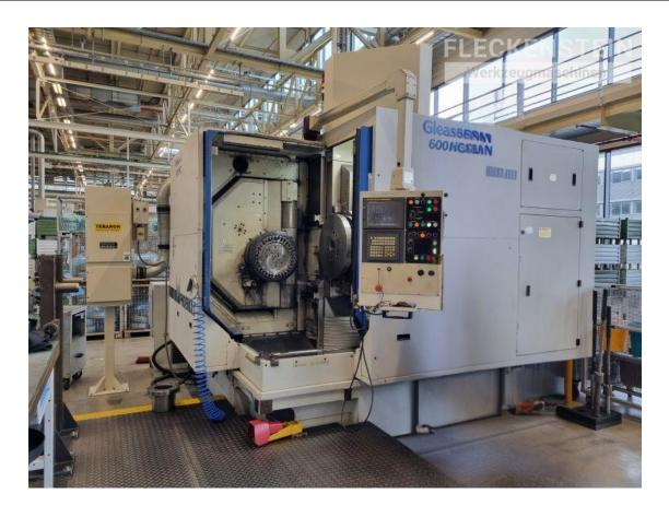
With the GLEASON PhoenixII® 600HC bevel gear cutting machine, manufacturers of medium-sized spiral and hypoid-toothed bevel gears can achieve faster cycle times and higher accuracies at lower workpiece costs.
